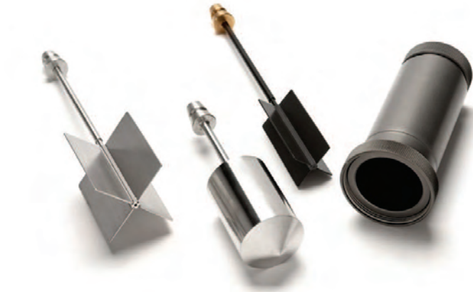
Figure 3: The different rheometer inserts (bob and vanes) and cup. N.B. the smaller vane was used here .
